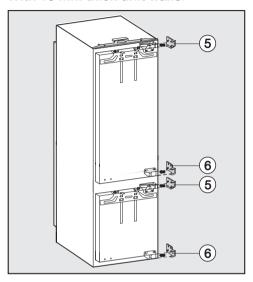
■ Clip spacers ⑤ onto the top hinges and spacers ⑥ onto the bottom hinges.
